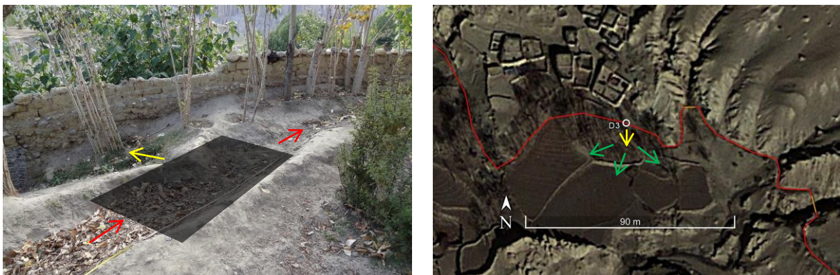
Figure 7.20: Position of the distribution chamber D3 ( x = 1882 m; 29^{\circ}05'44.51''N / 84^{\circ}00'03.79''E ). Left: The pipeline (red arrow) and the chamber (black rectangle) are proposed to be located on top of the open distribution channel (photo: 27/09/2013, Daniel Bernet). Right: Bird's eye view of the inspection chamber's location. The red line indicates the pipeline with gully crossings (orange sections), the yellow arrow highlights where the chamber's diversion pipe should meet the open channel network to distribute the water to the corresponding field area indicated by the green arrows (source: Google Earth Pro, accessed 30/01/2014).
