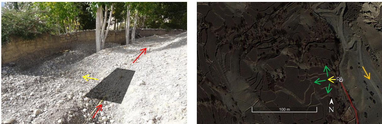
Figure 7.14: Position of the distribution chamber D2 ( x = 1475 \text{ m} ; 29^{\circ}05'36.57''\text{N} / 84^{\circ}00'07.71''\text{E} ). Left: The pipeline (red arrow) and the chamber (black rectangle) are proposed to be located at the illustrated position (photo: 27/09/2013, Daniel Bernet). Right: Bird's eye view of the inspection chamber's location. The red line indicates the pipeline, the yellow arrow highlights where the chamber's diversion pipe should meet the open channel network to distribute the water to the corresponding field area (green arrows). The path leading to Ghara is highlighted by an orange arrow (source: Google Earth Pro, accessed 30/01/2014).
