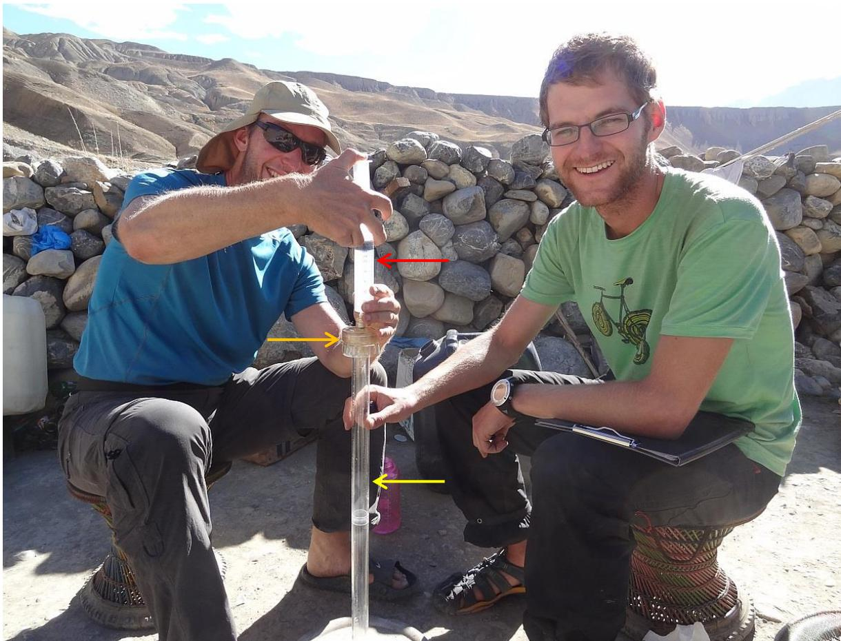
*Figure 10.10: Marco Baumer using the syringe (red arrow) to successively filtering the abstracted water with the graded filter paper inserted into the filter holder (orange arrow). Daniel Bernet is holding on to the turbidity tube with which the turbidity can be assessed visually (photo: 24/09/2013, Fidel Devkota).*
