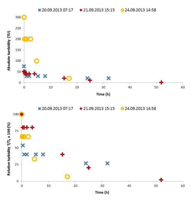
*Figure 10.12: Absolute (top) and relative turbidity (bottom) of the suspension stability test with samples taken on different days at different times.*
