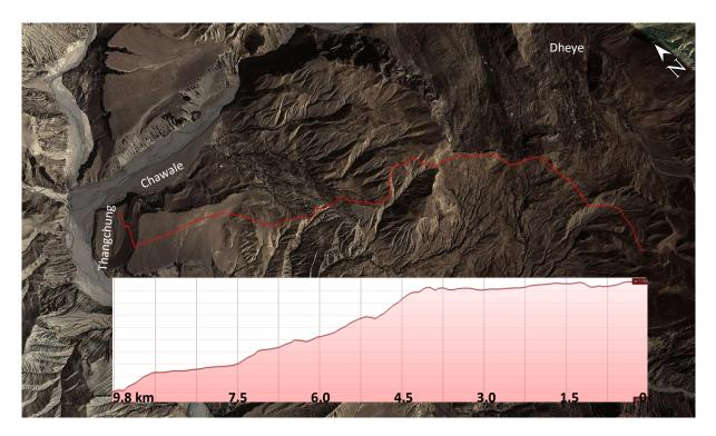
Figure 5.2: Possible routing of the pressure pipe transporting the water from the existing drinking water abstraction to Thangchung. The longitudinal profile of the pressure pipe created with Google Earth is indicated as well. The first roughly 4 km are sloped only slightly, thereafter the pipe is leading steeply down to Thangchung (source: Google Earth Pro, accessed 14/01/2014).
