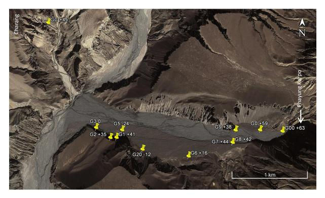
Figure 10.4: Illustration of the GPS measurement points with the indication of the relative elevation in relation to the point G3 located at the northern end of Thangchung given in meters. Note that these relative elevations are subjected to qualitatively assessed uncertainty ranges presented in Table 10.3 (source: Google Earth Pro, accessed 19/01/2014).
