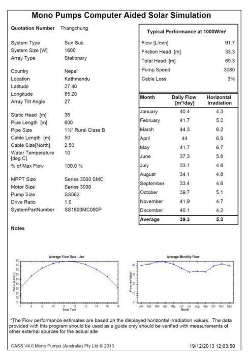
Figure 10.21: Calculation result of the CASS. The results show the capacity of one single solar pump powered by a 1600 W PV array. For the design, the minimal yield,  $33.1 \text{ m}^3/d$  in July, is relevant (source: CASS, Jeffery (2013)).
