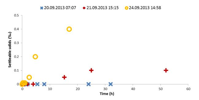
*Figure 10.13: Evolution of the settled solids' volume relative to the total abstracted water volume with increasing time the water is sitting still.*
