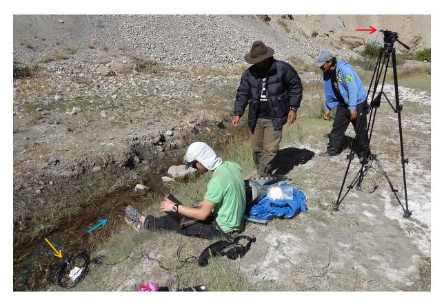
Figure 10.7: Daniel Bernet sitting next to Fidel Devkota and Pema Chewang who are assisting the experiment. The probe head of the conductivity meter is immersed in the water (orange arrow) and is sending the measurement values to the connected laptop. The flow direction is indicated by the blue arrow. On the right hand side the GPS antenna (red arrow) mounted on a tripod can be seen. With the GPS device the elevation of the spring could be approximated (photo: 24/09/2013, Marco Baumer).
