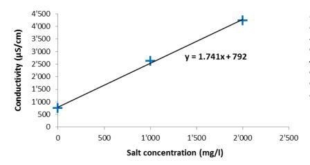
Figure 10.6: The function of the line of best fit gives the conversion factor (1.741) from salt concentration to conductivity. Additionally, the equation indicates the approximated conductivity of the raw water (792 mS/cm).
