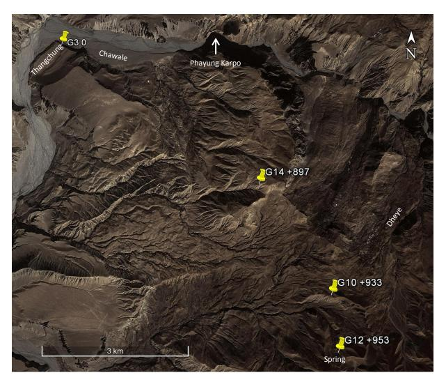
Figure 10.5: Illustration of the GPS measurement points, which were assessed in the context of the possible pipeline tapping the spring currently supplying drinking water to Dheye. The numbers beside the measurements' ID indicates the relative elevation compared to the point G3 located at the northern end of Thangchung. The associated uncertainty ranges, together with the coordinates, are presented in Table 10.3 (source: Google Earth Pro, accessed 19/01/2014).
