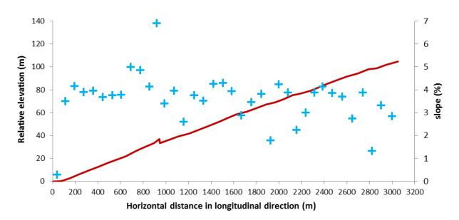
Figure 10.2: Longitudinal profile along the valley bottom from Phayung Karpo to the first section of the orchard. As can be seen from the profile, the valley bottom is quite evenly sloped. The tooth in the profile (red line) corresponds to the place, where the leveling jumped from the active riverbed onto the plain of Chawale. The scarp at this place is almost four meters high. The each section is indicated by the blue crosses.
