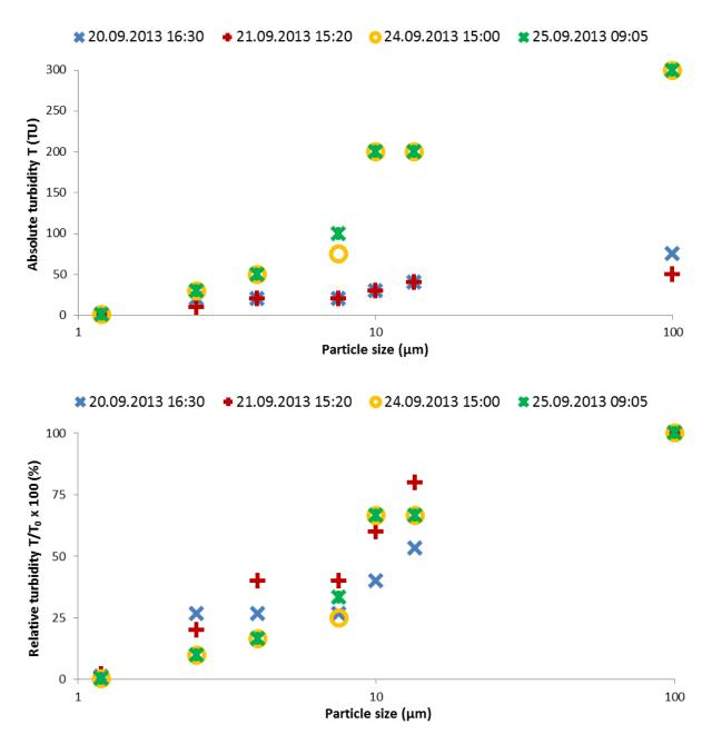
*Figure 10.11: Absolute (top) and relative turbidity distribution (bottom) of the filterability tests with samples taken on different days at different times.*
